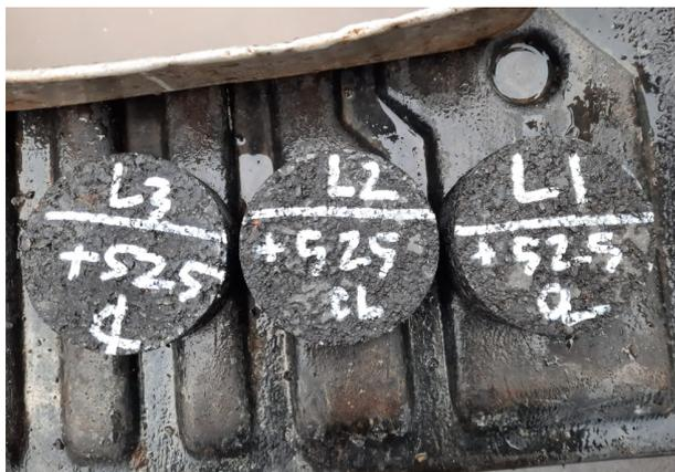
Benda Uji Core Drill
